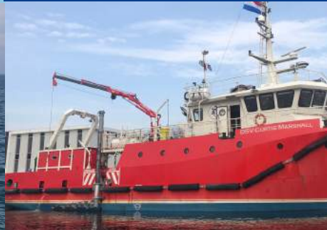
3 survey pole options which can be used to mount USBL transceivers, Sub Bottom profilers and Multibeam Sonars.
